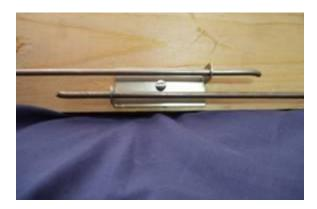
The rod that will attach to the right side of your fireplace opening needs to thread through the **left** side of the center bracket; the rod that will attach to the left side of your fireplace needs to thread through the **right** side of the center bracket (as seen facing your fireplace). The two rods are supposed to overlap, ensuring that the curtain can close all the way.
