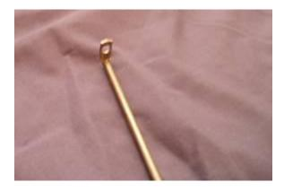
Both rods have a flat end; using a pair of vise grip pliers, very gently bend each flat end at a ninety degree angle. This will enable you to attach the rods directly to the side of your fireplace
